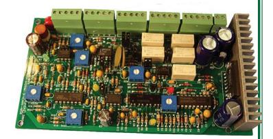
The OWNLINE input points connect to the CSPKR output points whenever the HC-0826 Intercom Amplifier is not INUSE. OWNLINE may be used as a substation of a remote intercom master to provide master to master communication. Multiple remote masters may be connected.
