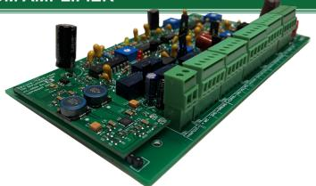
The OWNLINE input points connect to the CSPKR output points whenever the HC-0826 Intercom Amplifier is not INUSE. OWNLINE may be used as a substation of a remote intercom master to provide master to master communication. Multiple remote masters may be connected.
